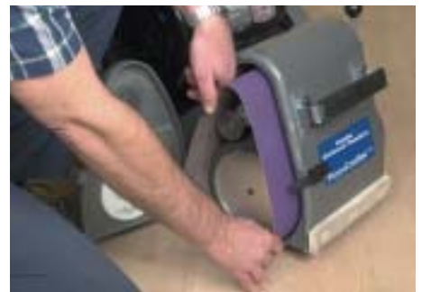
Recessed drum door provides better air seal and eases abrasive installation and adjustments
