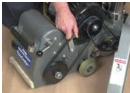
Quick release drive belt tension system eases disassembly and storage
